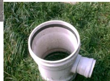
Tailrace Well—a standard 16x16x6 inch PVC Catch Basin. Installed under the Powerhouse, concrete is later poured inside the well, up to the point of exit to the 6 inch line.
