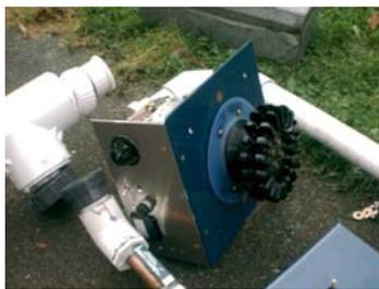
APM 3600 Pelton Wheel Turbine/Generator Sub-assembly. The turbine was built by Alternative Power & Machine of Grants Pass, Oregon.
